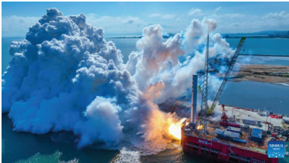
Tianlong-3 rocket first stage propulsion test
